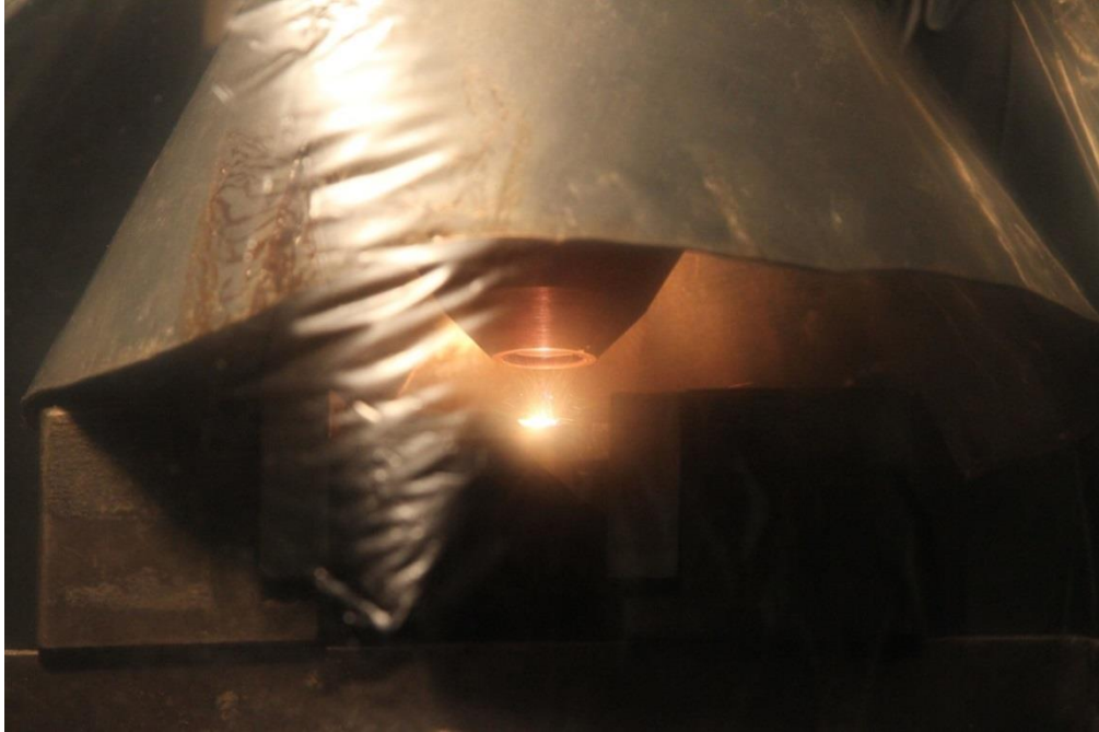
Figure 2.1. Deposition inside of a turkey bag.
