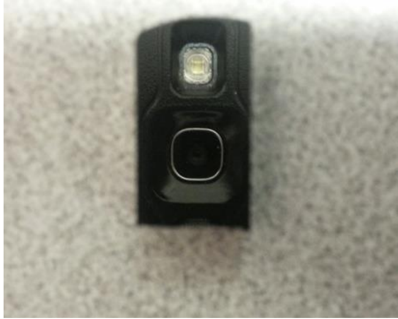
Figure 3.3. Coupon 21 after polishing. Note the reflection of the camera lens and flash bulb, indicating a mirror finish.
