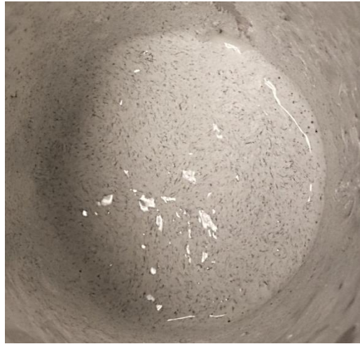
Figure 2.2. Paste with titanium fibers distributed in bioglass
