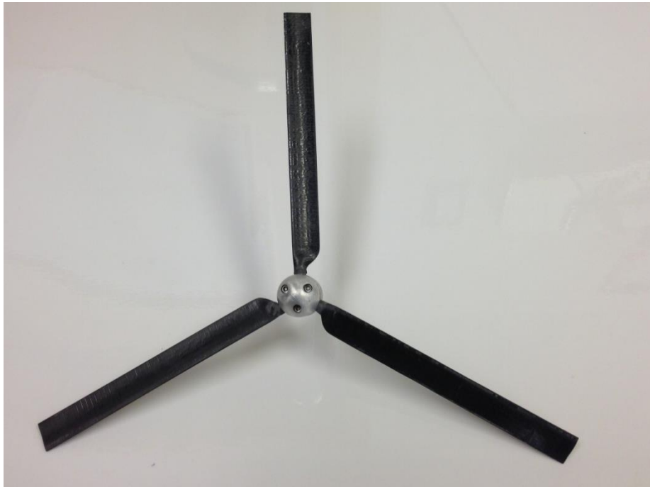
Figure 2.7. Front View of the Turbine Blades
