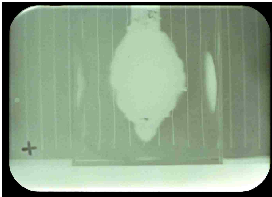
Figure 2.9 – Shockwave spallation occurring at 15% of typical burden
