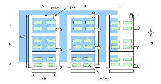
Figure 1. Small-plot design at Crowley during 2004: distribution of blocks (A, B, and C), plots (a, b, and c) and small rice areas.
