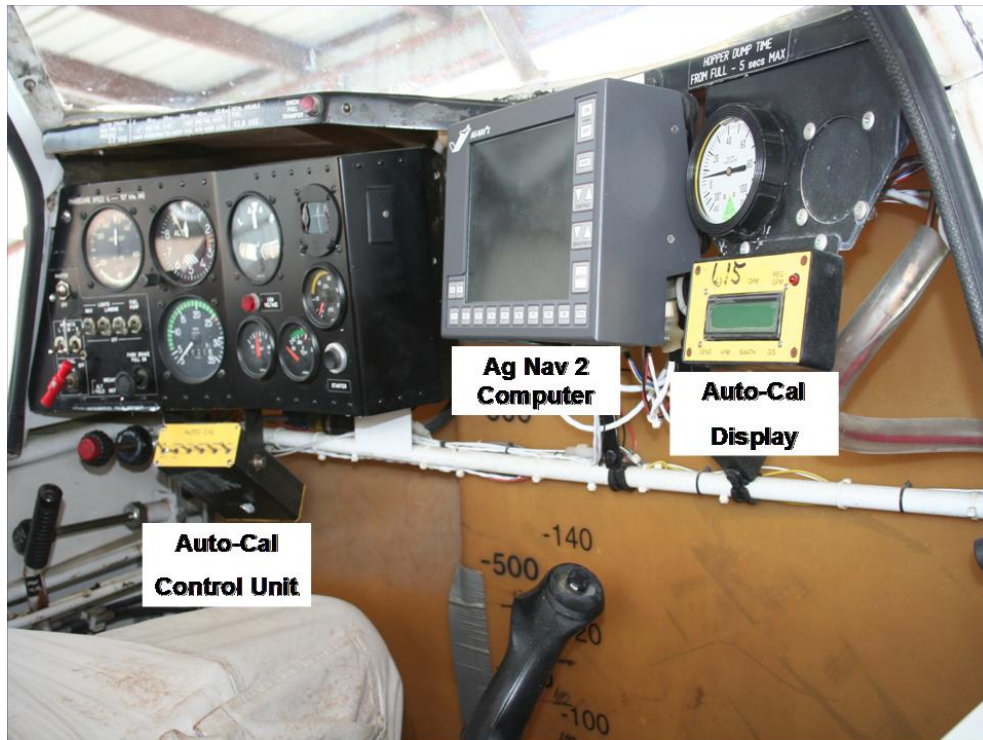
Fig. 9. View of the GA 200 aircraft console illustrating the flow control unit, calibration display, and on-board computer.
