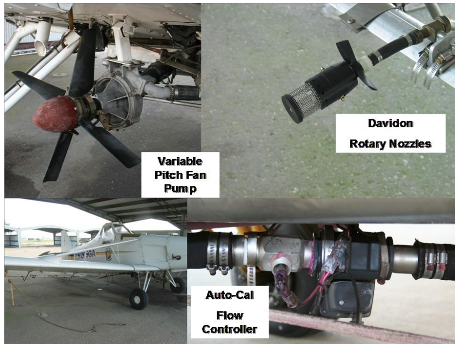
Fig. 10. External views of the GA 200 aircraft illustrating the variable pitch fan pump, rotary nozzles, and Auto-Cal flow controller.
