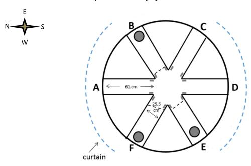
Figure 7. Schematic of the radial arm water maze. Dotted lines across arms indicate hanging fishing line. Grey boxes at the entrance to each arm indicate where gauze was placed. Grey circles at the end of an arm indicate where an escape platform was located. Arms containing escape platforms were scented via extract applied to the gauze. Visual spatial cues (see Figure 8) were affixed to the center of the each curtain.
