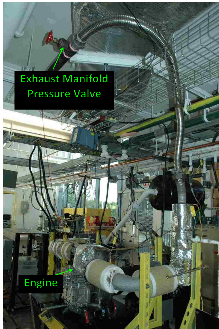
Figure 3.4. Exhaust piping – exhaust manifold back pressure valve
