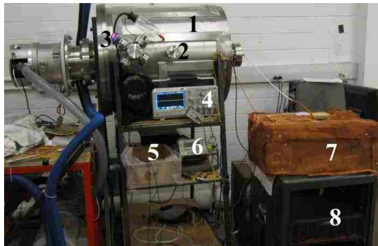
Figure 2.8: 1. Vacuum Chamber; 2. BNC-BNC Passthrough; 3. Lesker Pressure Gauge; 4. Tektronix DPO 2024 Oscilloscope; 5. Op-Amp Integrator Circuit; 6. Rigol Function Generator; 7. Faraday Cage; 8. Crown Amplifier.
