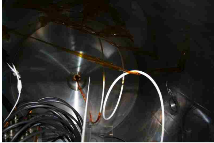
Figure B.2: Special care must be taken to insure that arcing does not occur between the high voltage wire and the vacuum chamber walls.
