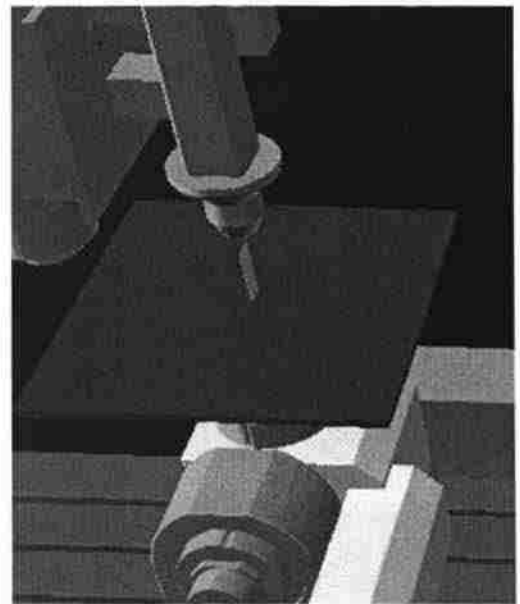
Figure 15. Illustration of the Overhang Part Deposition in Layers
