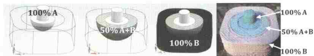
Figure 21: Demonstration of fabricating a functionally graded material part using two \text{CaCO}_3 pastes of pink and blue colors.
