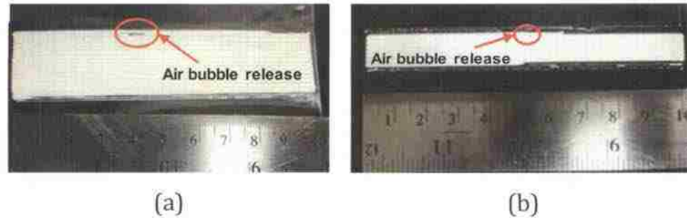
Figure 16: Parts with gap defects caused by an air bubble release for (a) velocity controller with u_{ref} = 0.01 mm/s and (b) extrusion force controller with F_{ref} = 630 N.
