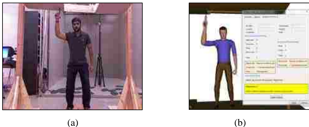
Figure 4.26. RULA: (a) posture in real world and (b) simulation in Jack showing Analysis Summary tab of RULA tool
