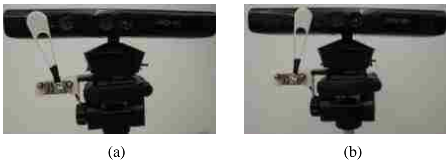
Figure 3.11. Shutter positions (a) open and (b) closed
