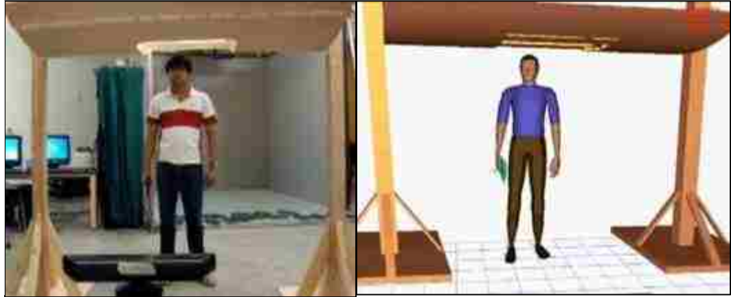
Figure 4.14. Simulation of fastening operation using a Kinect sensor, column 1: sequence of snapshots showing a person performing fastening operation, and column2: the corresponding simulation snapshots in Jack (cont)
