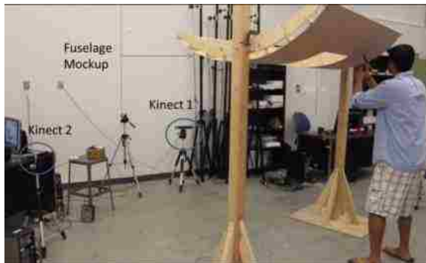
Figure 4.21. Set-up for two-Kinect system
