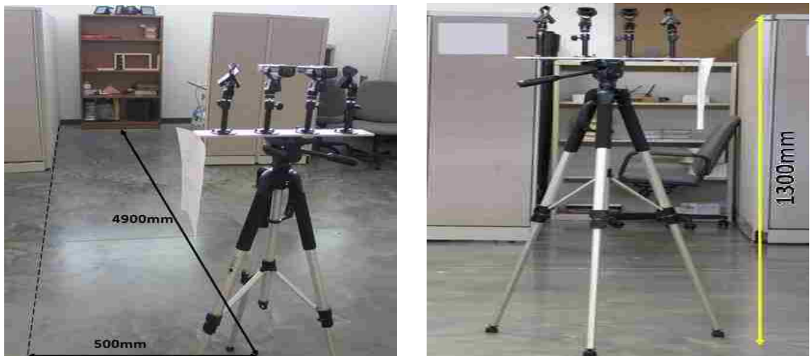
Figure 6.4. Positioning the Stereo Camera System for Tracking
