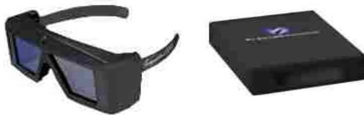
Figure 2.5. Shutter Glasses and Infrared Emitter
