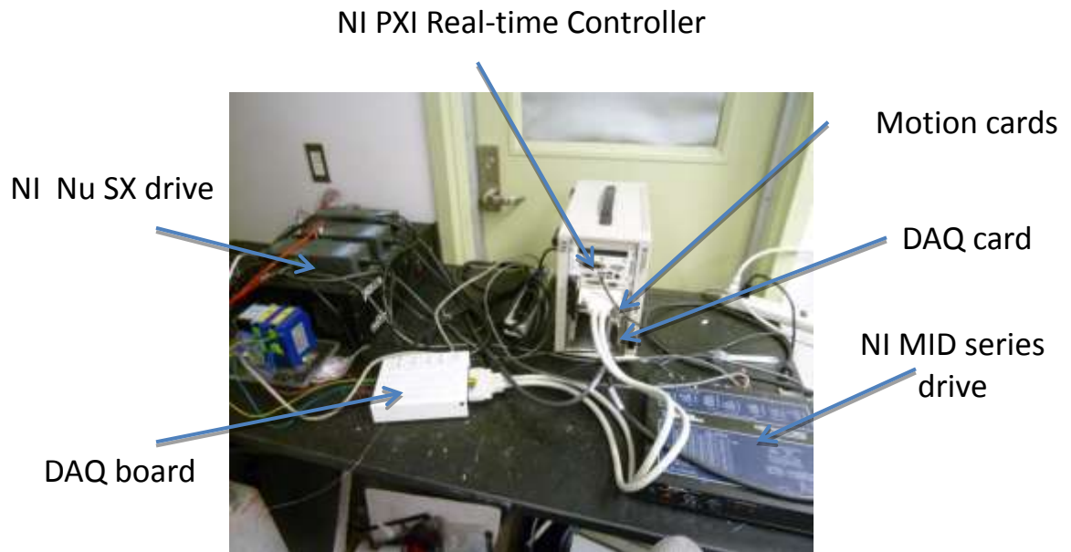
Figure 2.2. PXI NI N1011 chassis with real-time controller, two NI drives, two motion cards, one DAQ card, and one DAQ board
