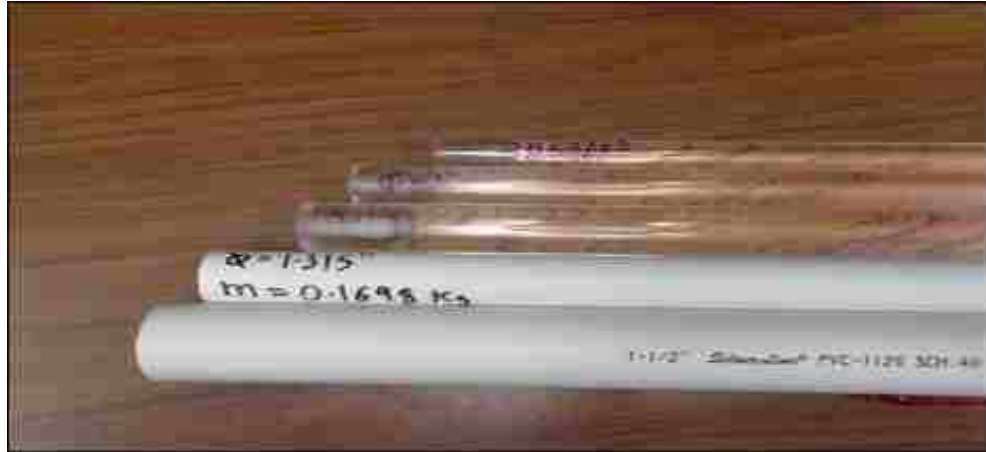
Figure 4.5. Different diameter cylinders used in the experiment
