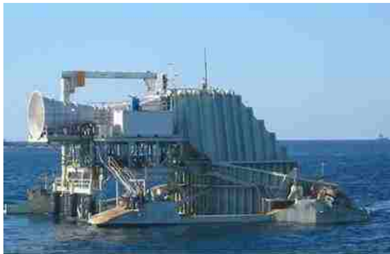
Figure 1.3. Energytech's Oscillating Water Column [9]
