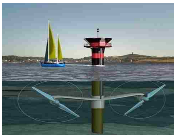
Figure 1.12. ‘Seagen’ twin rotor turbine in Strangford Lough [17]
