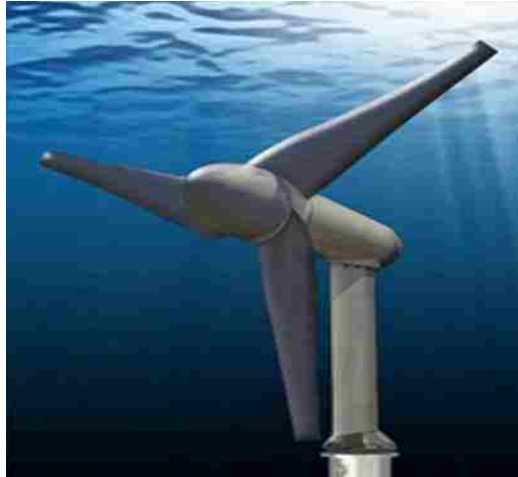
Figure 1.11. Three blade horizontal axis turbine by Verdant Power [15]
