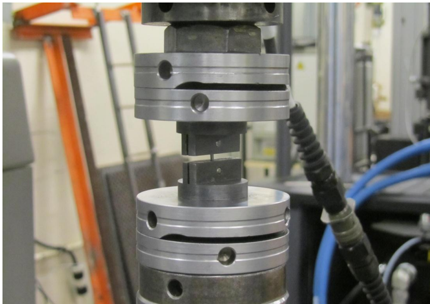
Figure 2: Testing set-up for tensile test for miniature size specimens
