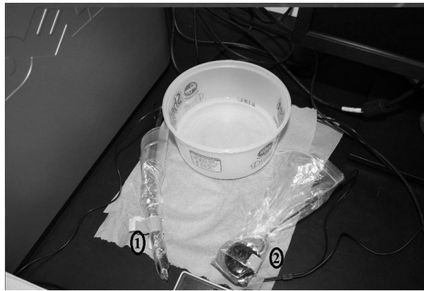
Figure 2.2. Headphone(1) and microphone(2) with waterproof 'enclosures'
