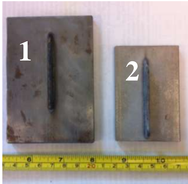
FIG. 10. DEPOSITS ON SUBSTRATES WITH A LARGE \xi_{sub} VALUE (1) AND A SMALL \xi_{sub} VALUE (2).
