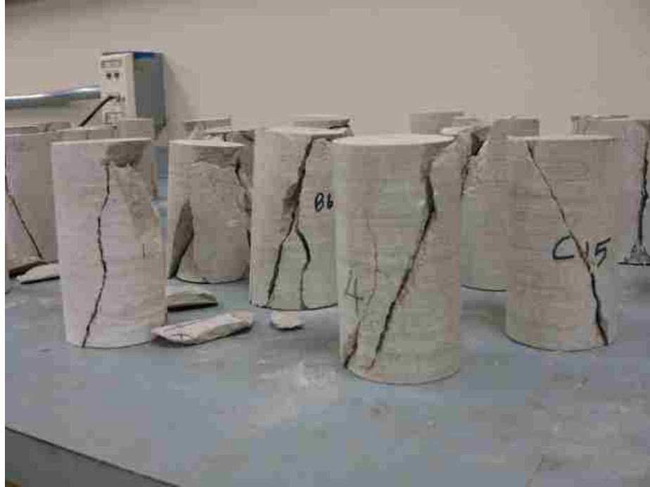
Figure 3.9. Failure mode associated with Indiana limestone
