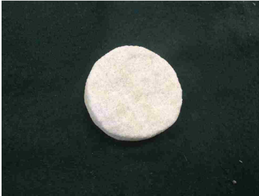
Figure 3.2. The best sample obtained from the coring operation (a disk with the thickness less than 25mm.)
