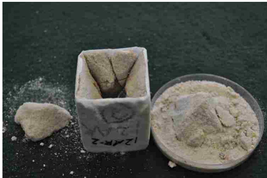
Figure 4.30. Failure formation associated with specimen 12AR -2.
