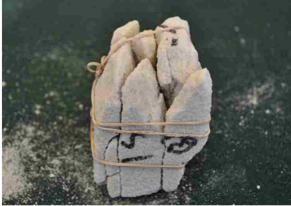
Figure 4.34. A typical specimen appearance after the uniaxial compression test
