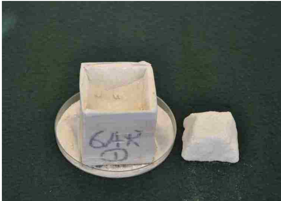
Figure 4.32. Failure formation associated with specimen 6AR-1.
