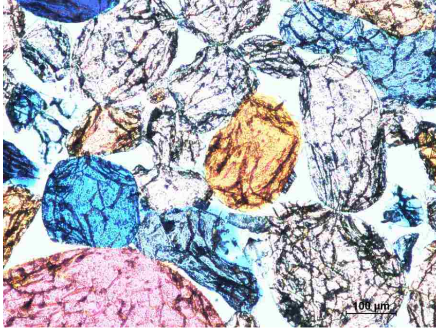
Figure 6.5. Stress trajectories and a highly stressed small sand grain.
