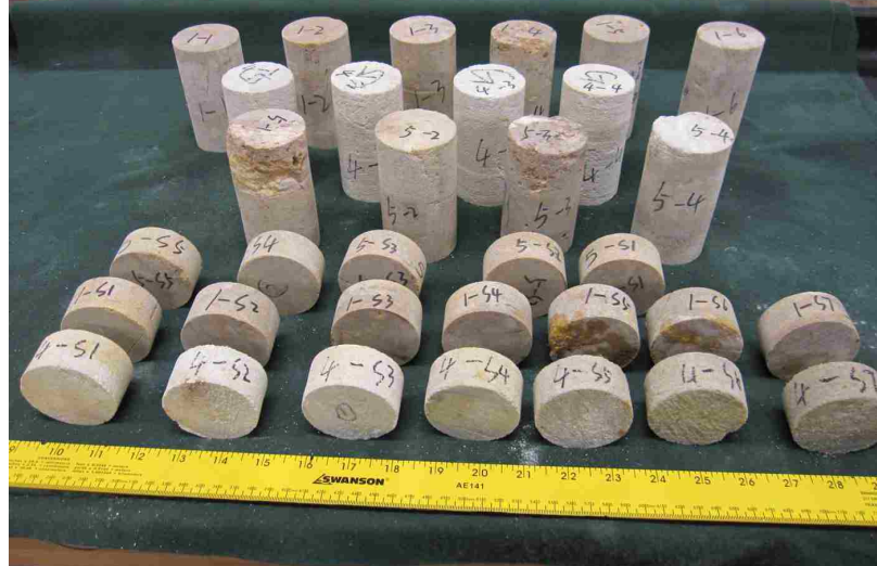
Figure 3.18. Specimens of cemented St. Peter Sandstone
