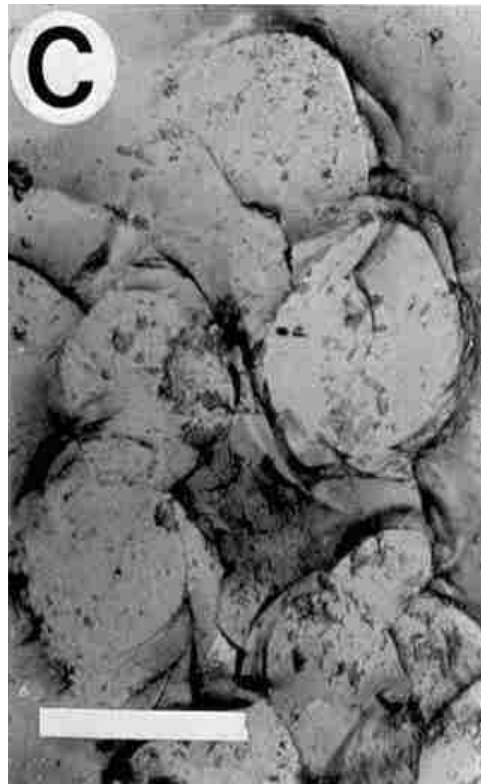
Figure 6.12. Full-circle Hertzian cracks formed on a quartz sand grain under experimental eolian conditions in a NASA wind tunnel. Scale bar equals 10 microns (Johnson et al., 1989).
