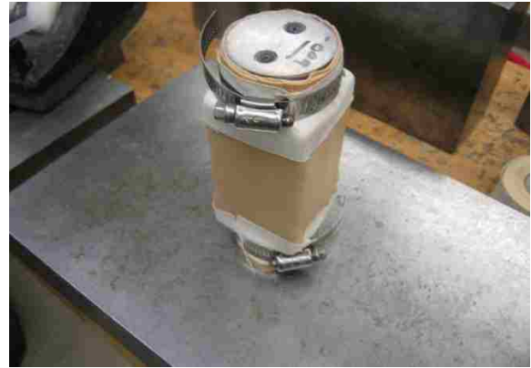
b) Seals along loading platens
