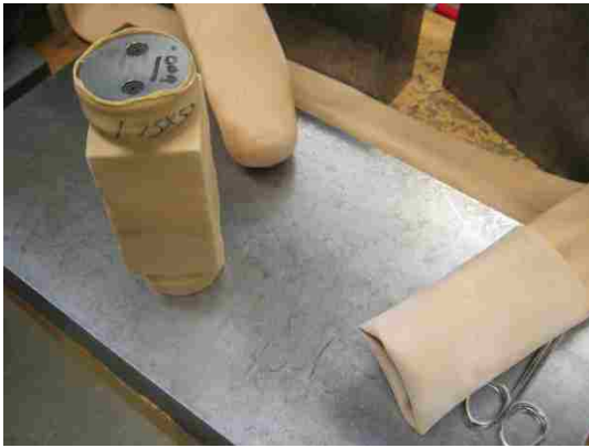
a) Specimen assembly in latex jacket
