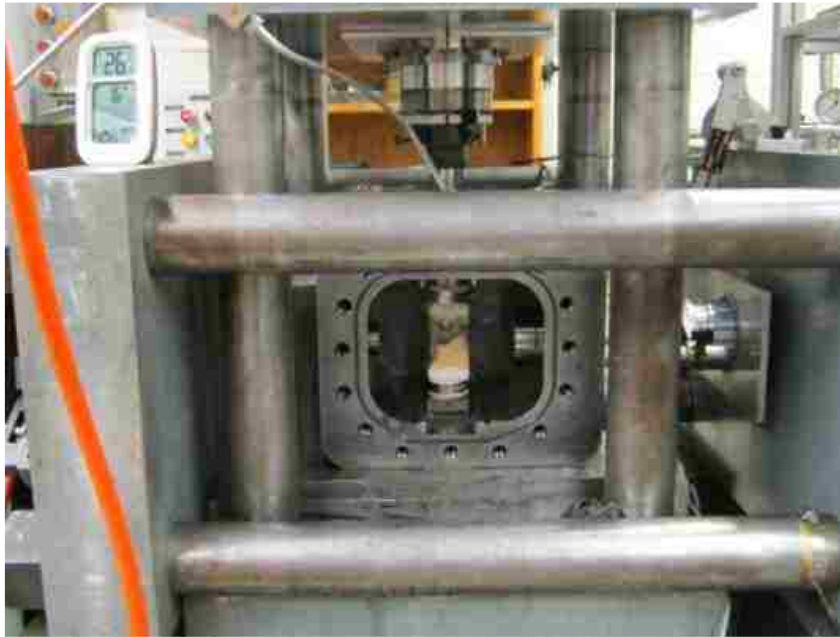
Figure 4.11. The triaxial test apparatus utilized for this investigation
