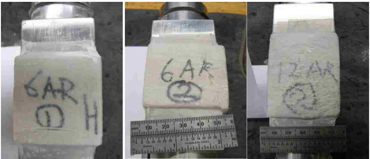
Figure 4.29. Specimens after the triaxial test.
