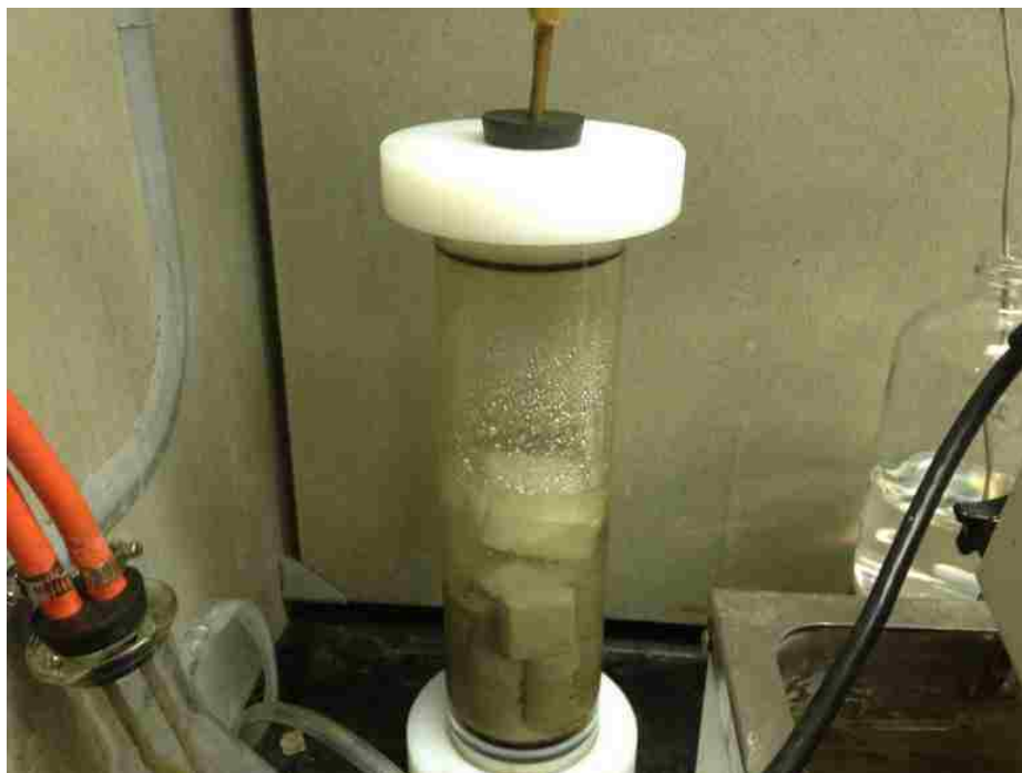
Figure 5.6. Samples are saturated by fluid immersion in a vacuum using liquid saturation method.
