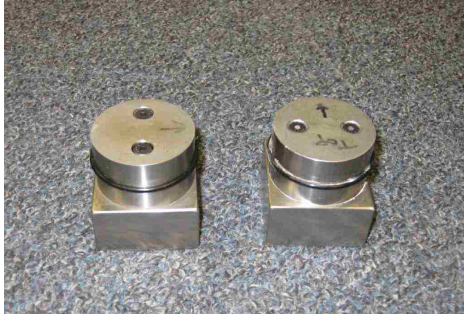
Figure 4.13. Two loading platens, which allow the drained condition test, were specially designed and manufactured for this research.
