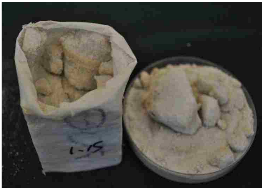
Figure 4.33. Failure formation associated with specimen 1S-1.
