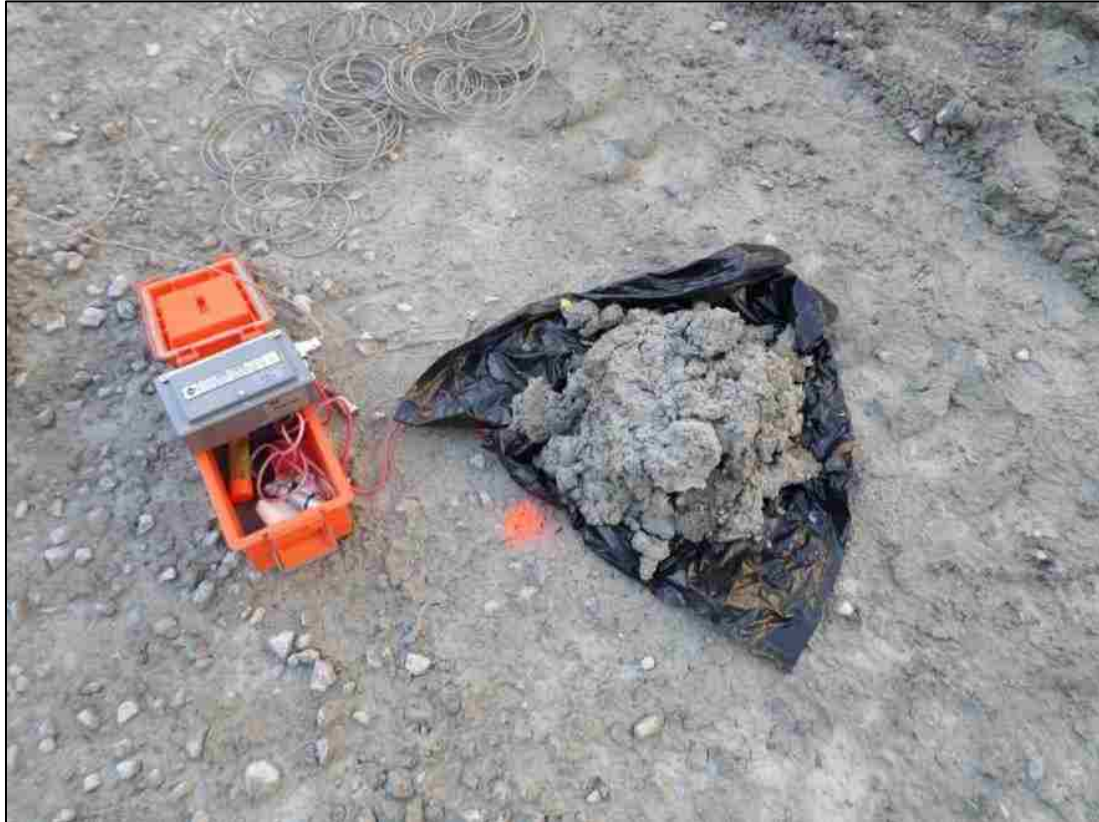
Figure 3.4. Mini-Seis x2 geophone coupled to the pit floor using a mud cap.
