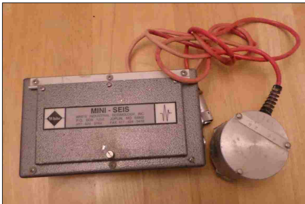
Figure 3.1. Mini-Seis x2 model manufactured by White Industrial Seismology.
