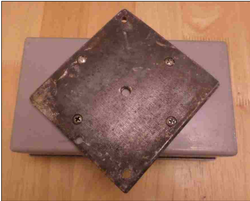
Figure 3.2. Steel plate mounted to the bottom of the Mini-Seis x1 seismographs.
