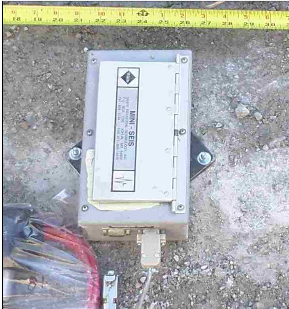
Figure 3.3. Mini-Seis x1 seismograph mounted to the quarry floor.
