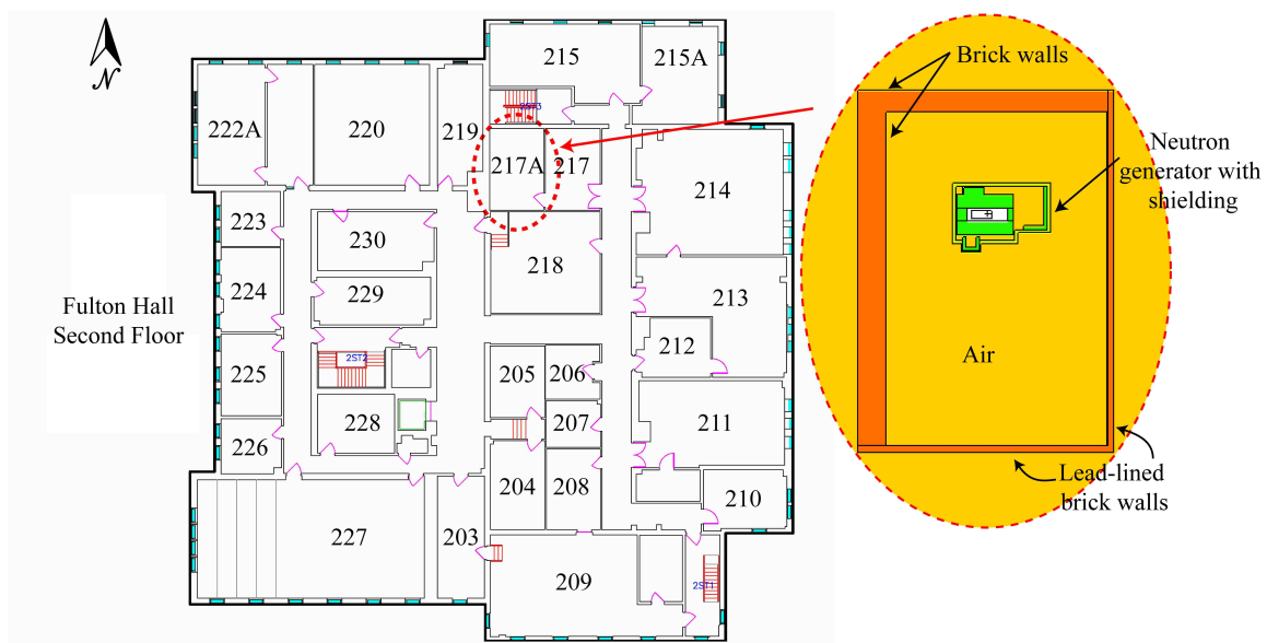
Figure 1.2 Layout of second floor of the Fulton building where the generator is located. Also shown is a zoomed image of the room (217A) where the generator is installed.
