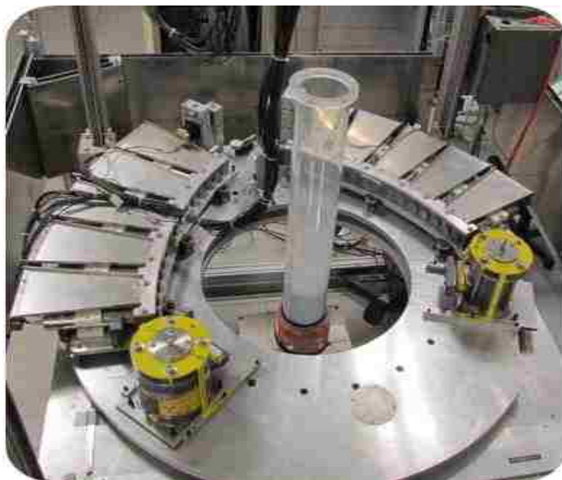
Fig. 3. Photograph of the DSCT technique, and 6-inch spouted bed inside the setup for scan.
