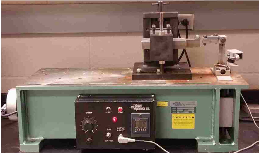
Fig. 2. Bending fatigue equipment.
