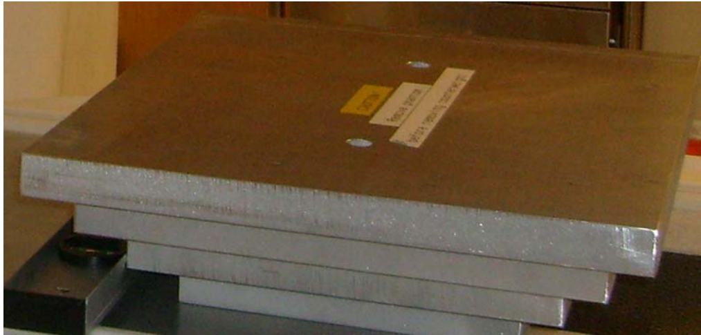
Figure 6.6 A series of counterweights were used to balance the heavy phantom on the phantom holder.
