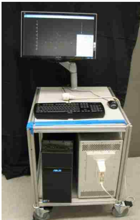
FIGURE 5.2: Photo of the second generation clinical device. The Verasonics® Ultrasound Engine (in silver on the right) and ultrasound transducer (P4-1 shown in front of the keyboard) is used to both image and move stones. The PC (on the left) communicates with the Verasonics via MATLAB® software.
