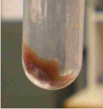
FIGURE 2.13: Photo showing the tissue sample in the bottom of a pipette. The pipette will act as a container to recirculate the tissue as is predicted to occur in bulk boiling histotripsy.
