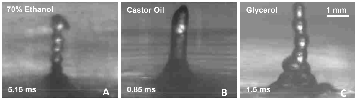
FIGURE 4.8: Frames taken from the high speed videos of A) 70% ethanol at a 180 W/cm 2 acoustic intensity, B) castor oil at a 24,000 W/cm 2 intensity, and C) glycerol at a 24,000 W/cm 2 intensity. In ethanol (A), the intensity was just above its atomization threshold; on the upper left just under the “70% ethanol” label, you can see a droplet that was ejected from the fountain. In both castor oil (B) and glycerol (C), the intensity was at the maximum output of the transducer and atomization did not occur ( i.e. no droplets were emitted from the fountain).
