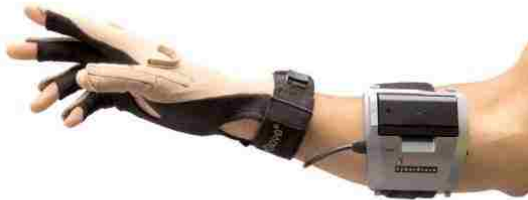
Figure 18 – CybergloveII dataglove used to record joint angles
