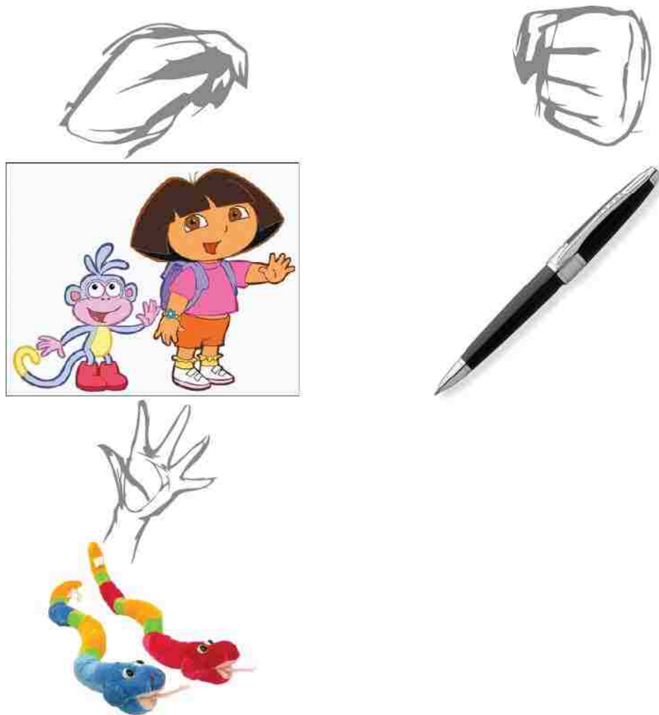
Figure 9 – Objects presented to the subject included a 6cm x 6cm picture of cartoon character “Dora the Explorer”, a ball point pen, and a stuffed toy snake. Each was presented to the subject in such a way as to induce a 4-finger opposed prismatic grip, power grip, and gross envelopment grip, respectively.
