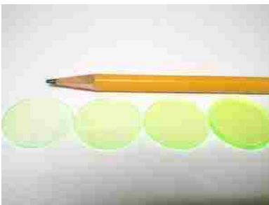
Figure 8 Photo representations of dye-in-polymer.
