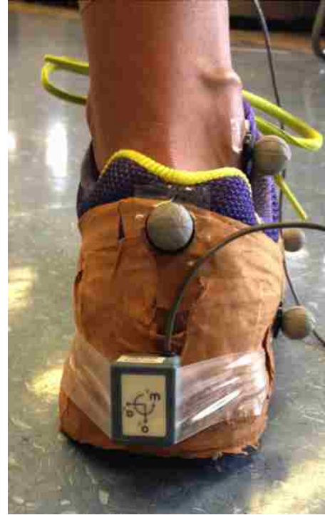
Figure 3.5: Sensor used to collect acceleration of right foot.
