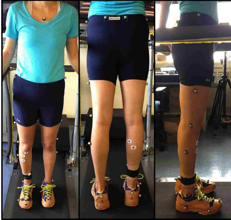
Figure 3.6: Retro-reflective marker (silver balls) placement on subject, surface electrodes (white rectangles) and acceleration monitoring unit (secured on medial right tibia with black strap) placement also shown.
