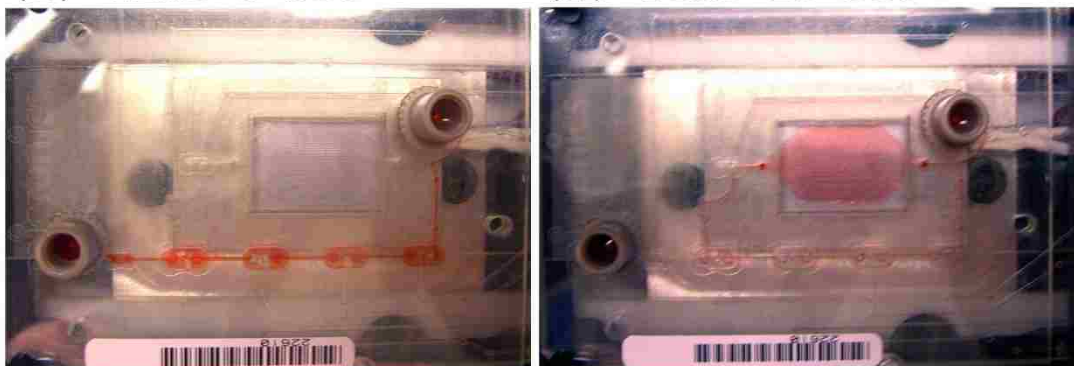
Figure 42 – Recirculation of sample in the microfluidic platform. At time 0, red liquid has been loaded into the pump line, and clear liquid into the imaging chamber (left). Upon starting the execution of the on-card pumps, the sample is recirculated (right). Photo courtesy of Joshua Thompson.
