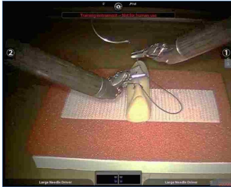
Figure 26 - Criterion video of a surgeon performing an FLS intracorporeal suturing task using the da Vinci surgical robot.
