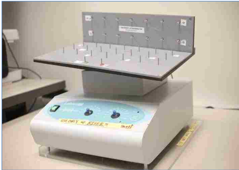
Figure 4 - Rocking pegboard was mounted to a lab mixer rotating at 8 cycles per minute.
