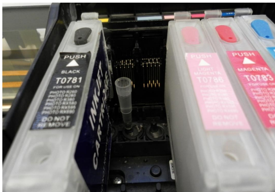
Figure 19. A pipette tip reservoir was fabricated by truncation of a 200 \mu\text{L} pipette tip so that the tip could be inserted onto the printhead. During printing preparation the reservoir is filled with either priming or bio-ink solution.
