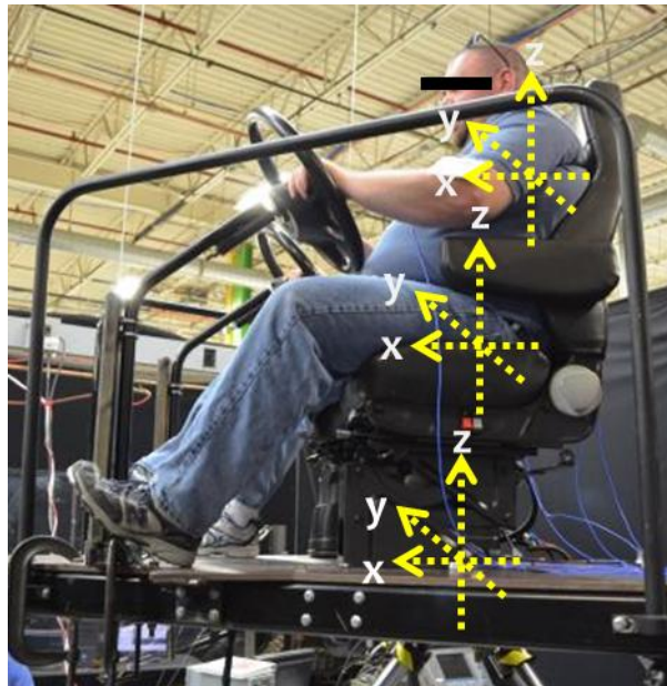
Figure 2.3 Shaker table experiment setup. Locations of arrows mark approximate placement of three accelerometers (image courtesy of Ryan Blood).
