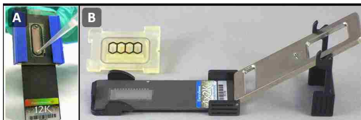
Figure 14. (A) The single chamber flow cell is clamped against the chip using plastic clips on either side. (B) The four-chamber flow cell requires a clamping structure to secure it in place.
