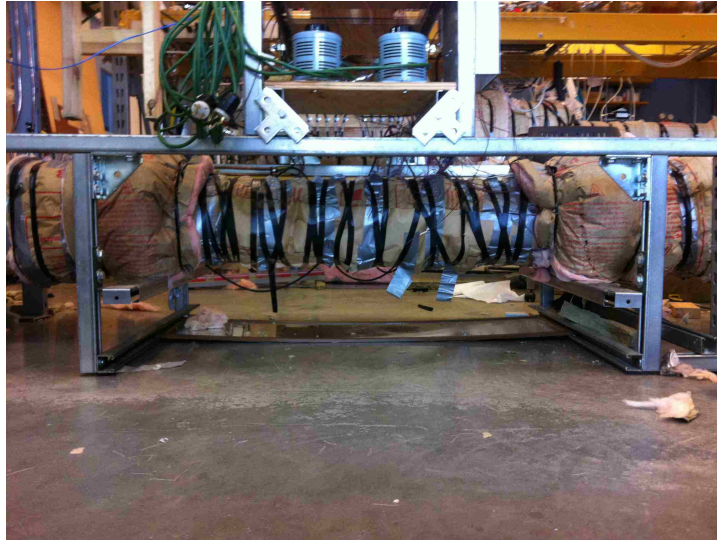
Figure 3.28: Fully insulated air test section.
