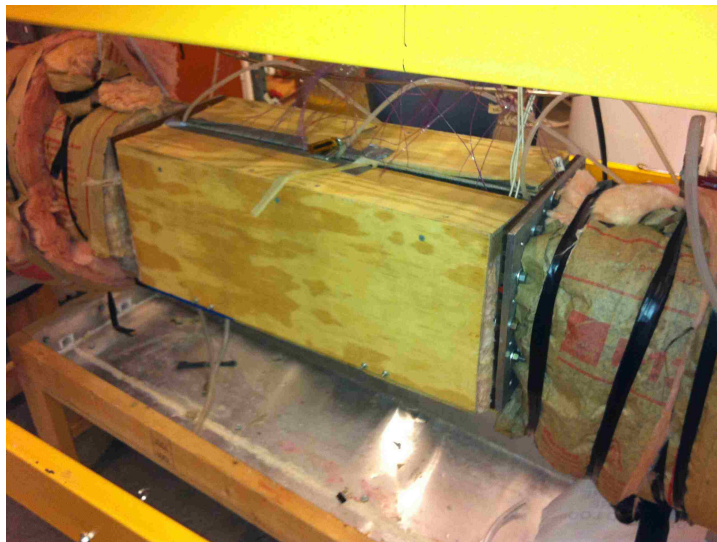
Figure 3.11: Mineral wool insulation around liquid test section.
