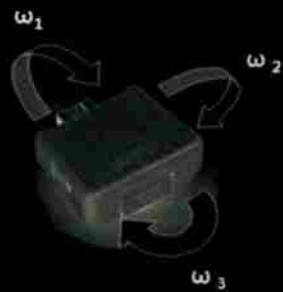
(a) Wii MotionPlus Accessory ( \omega_1, \omega_2, \omega_3 are angular velocities along three major axes of rotations)
