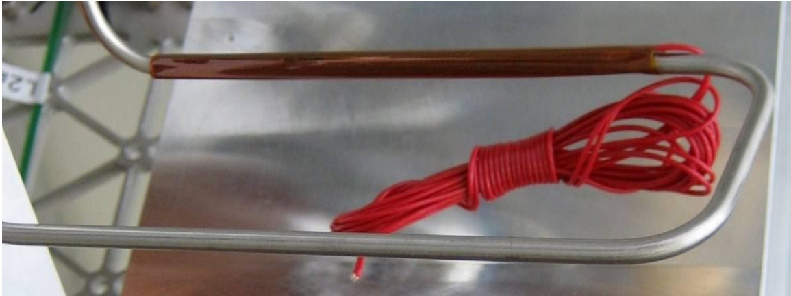
Figure 3.16. Line Heater Attached to Tubing
