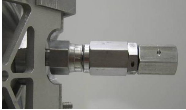
Figure 5.8. Panel Cut-out for Fill Valve
