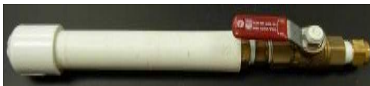
Figure 4.2. Immersion Capsule for R-134a Compatibility Testing
