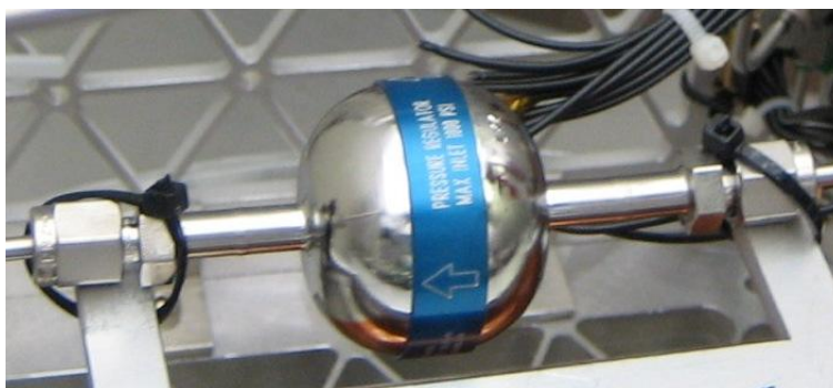
Figure 3.11. HFS3B Regulator Integrated into MR SAT
