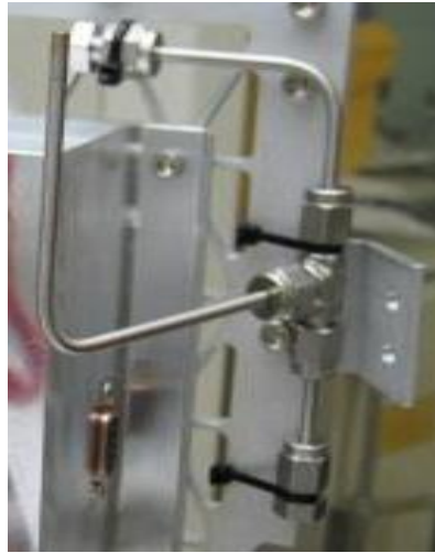
Figure 3.12. Propellant Line and a Swagelok Fitting
