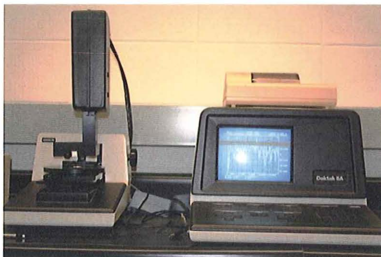
Figure A1.1. Sloan Dektak IIA Surface Measuring System. Dektak IIA components: Console: bottom right, Printer: top right, Scanning Head, left.
