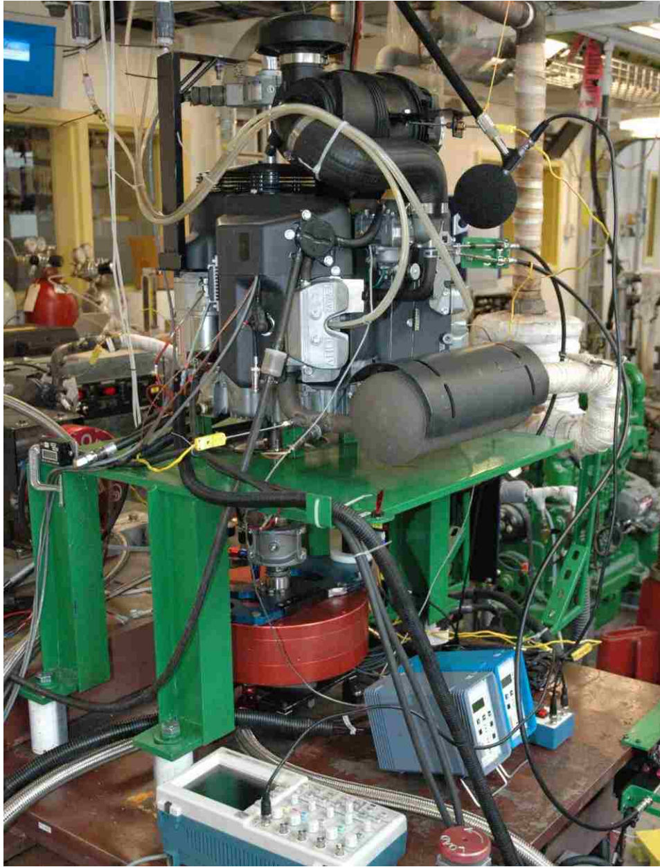
Figure 2.1: Test engine stand with associated instrumentation
