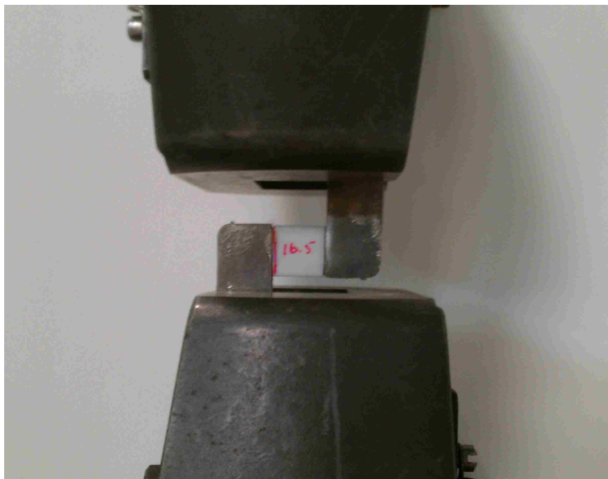
3.18. Shear Test Setup. The aluminum L brackets are clamped into the grips used for tensile testing.
