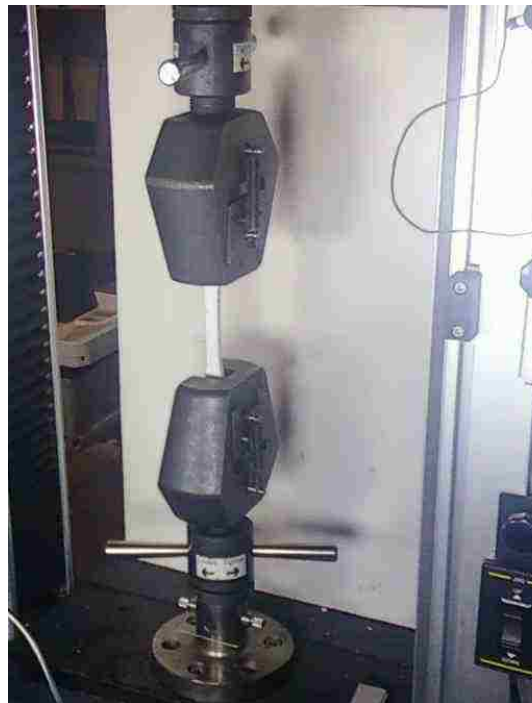
Figure 3.2. Tensile Test Setup. A dogbone specimen is loaded into the Instron material testing machine via two clamps. The lower clamp is stationary and the top clamp is fixed to a load cell mounted on a computer actuated beam. This beam raises and lowers depending on the type of test being conducted.
