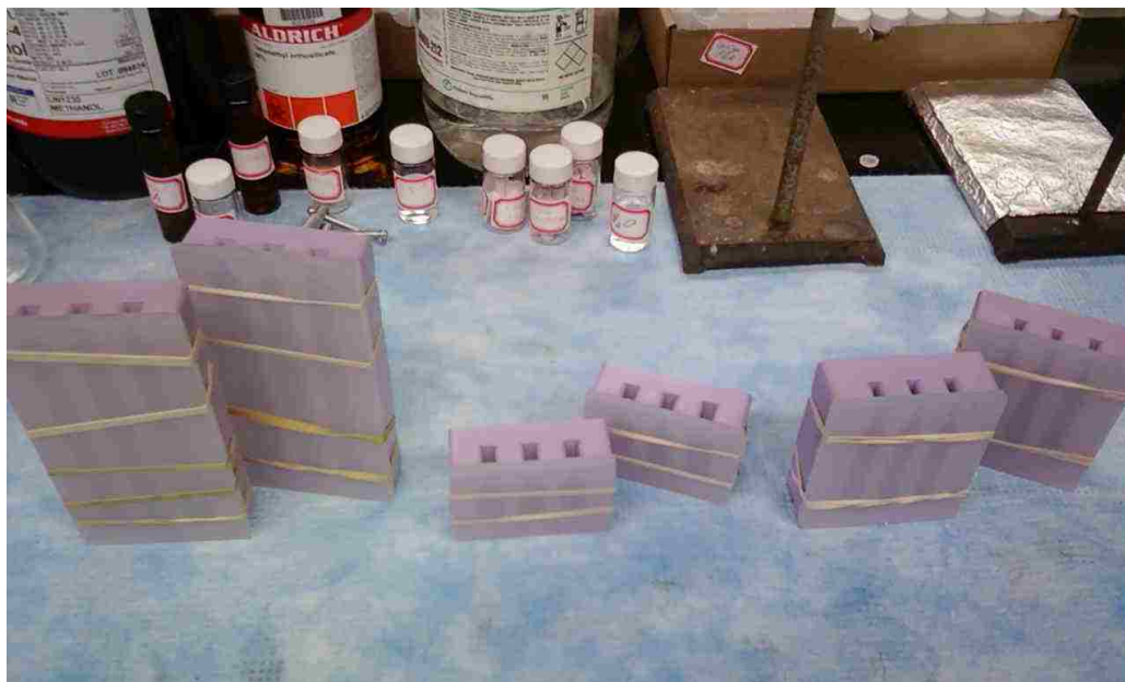
Figure 2.3. Finished Silicone Molds. To complete the molds a sheet of polypropylene plastic is fixed to the open face of the silicone molds with rubber bands. This method allowed quick and easy access to samples after they had formed wet gels.
