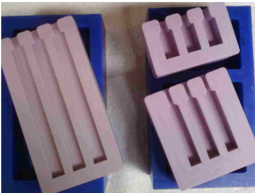
Figure 2.2. Silicone Molds After Release from Wax Blocks. After being left to cure overnight the (now solid) silicone is removed from the wax blocks. The cured silicone is solid but flexible, allowing easy removal of delicate PUA samples.
