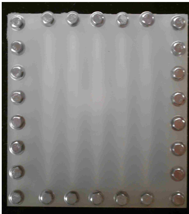
Figure 2.7. Assembled Polypropylene Mold. Polypropylene sheets have been stacked and bolted together. Openings are left at the top through which solution is poured. Here the outline of the mold cavity is partially visible, revealing the dogbone shape used for tensile testing.
