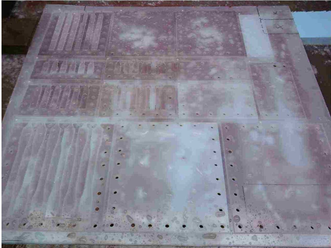
Figure 2.6. Freshly Cut Polypropylene Sheet. A computer controlled routine was created to cut the required mold-making parts from polypropylene plastic. These parts will be stacked and bolted together to form the new molds.
