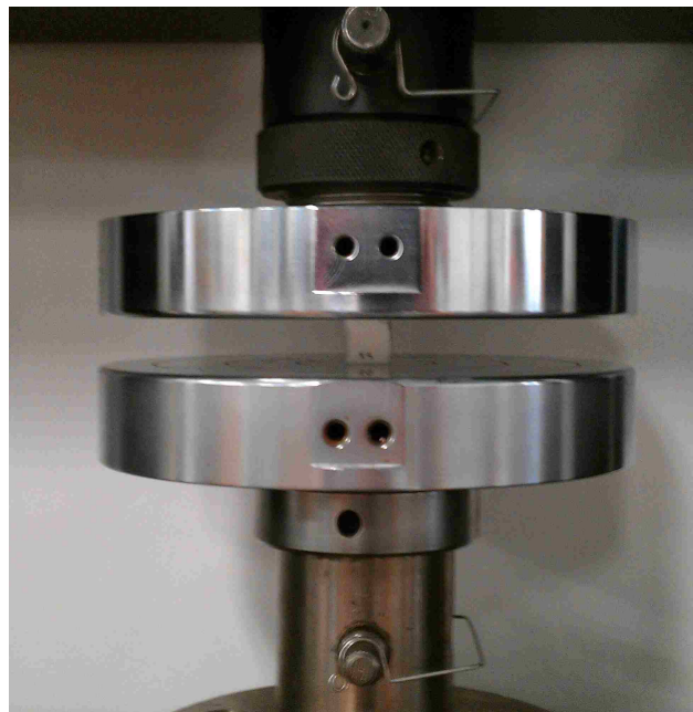
Figure 3.6. Compression Test Setup. The Instron testing machine has been fitted with two plates, one being fixed to a load cell, for the compression tests.
