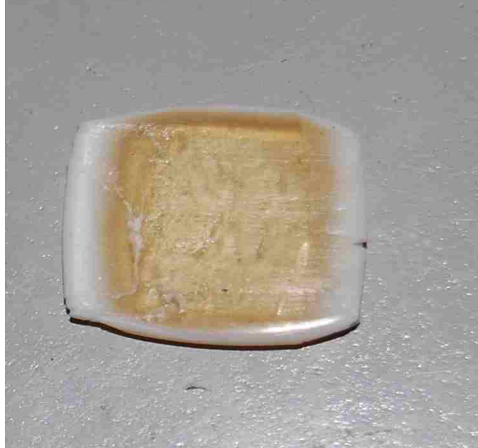
Figure 3.11. Compressive Test Specimen After Testing. The specimen has been compacted to approximately 10% of its original height. Plastic deformation to this extent has reduced the size of the gaps between adjacent microstructures leaving the material semi-translucent. A few cracks are evident, though the specimen remains intact.
