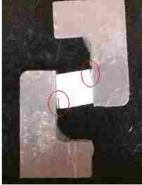
Figure 3.21. Failed Shear Sample. The above figure shows the fractures in the sample (circled in red) shortly after testing.
