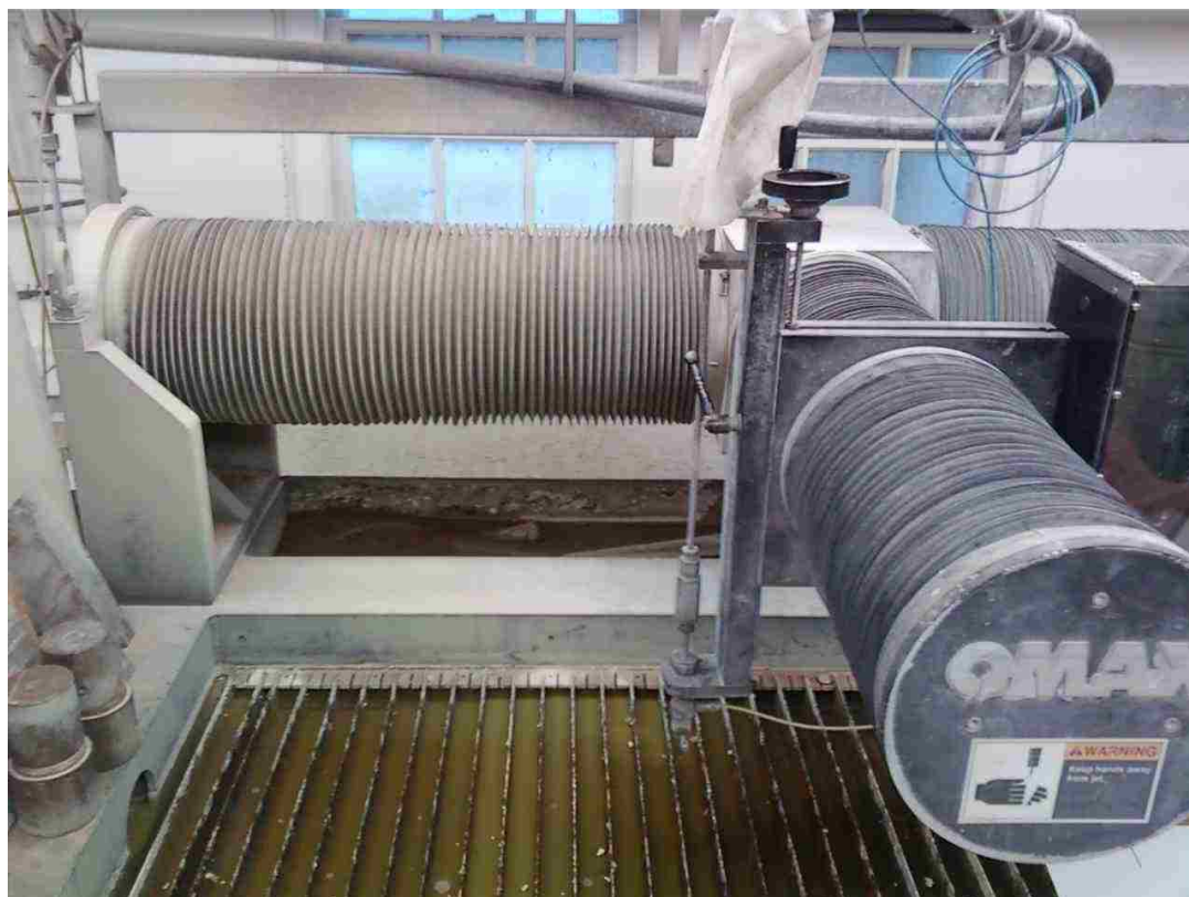
Figure 2.5. Missouri University of Science and Technology Waterjet. High pressure water is fed through a computer controlled nozzle to machine parts a variety of materials including metal, wood, plastic, and stone.
