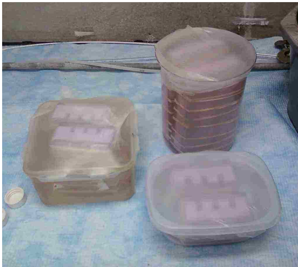
Figure 2.4. Silicone Molds in Acetone Bath. Due to shrinking of the PUA samples within the silicone molds (caused by the absorption of acetone from the samples into the silicone) the entire assembly was soaked in acetone prior to and during gelation of PUA.
