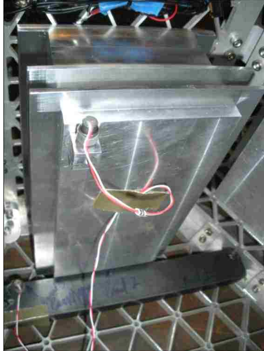
Figure 4.10. Accelerometer Mounted to the Battery Box on MR SAT Panel 2
