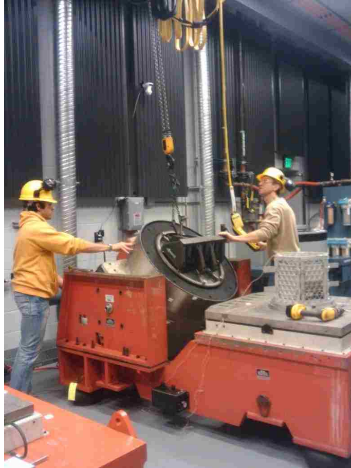
Figure 4.4. Rotating the Shaker Table for X- and Y-Axis Tests
