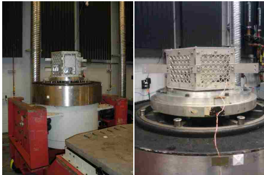
Figure 4.3. MR SAT (Left) and MRS SAT Shown Mounted to the Shaker Table
