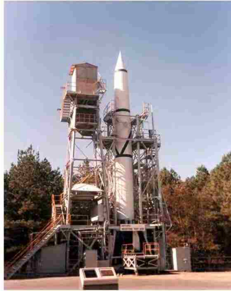
Figure 1.1. First Rocket Test Stand Used in Vibration Testing [9]
