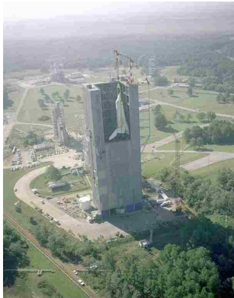
Figure 1.4. Space Shuttle Enterprise in the Dynamic Test Stand [13]
