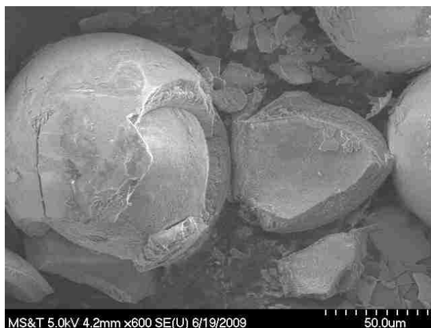
Figure 3.11: SEM image of partially reacted CaLB3-40-MoSci microsphere (0.25 M K_2HPO_4 , pH=12, 37°C, 2 days).
