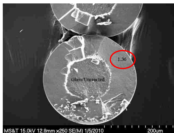
Figure 3.26: Partially reacted CaLB3-40-S50 microspheres in 0.5 M phosphate solution at 37°C for 6 days. The reacted shell has a Ca/P value of 1.43, 1.53, 1.41, and 1.36. The Ca/P value for the unreacted glass core is 4.41 (Contd.).
