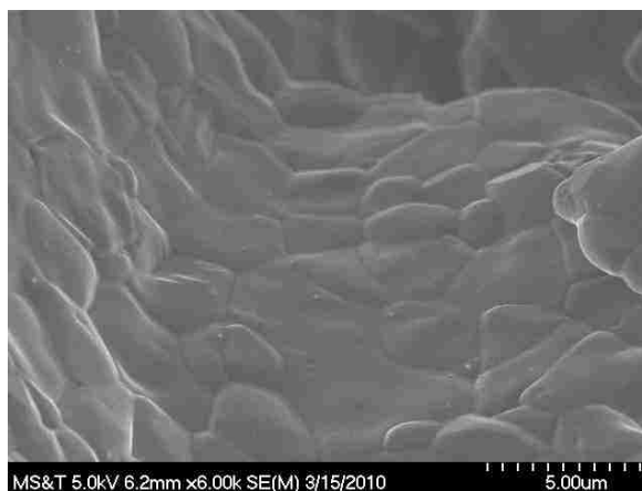
Figure 3.44: Internal microstructure of as-reacted CaLB3-40-S50 microspheres heat treated at 1200°C for 1 hour.
