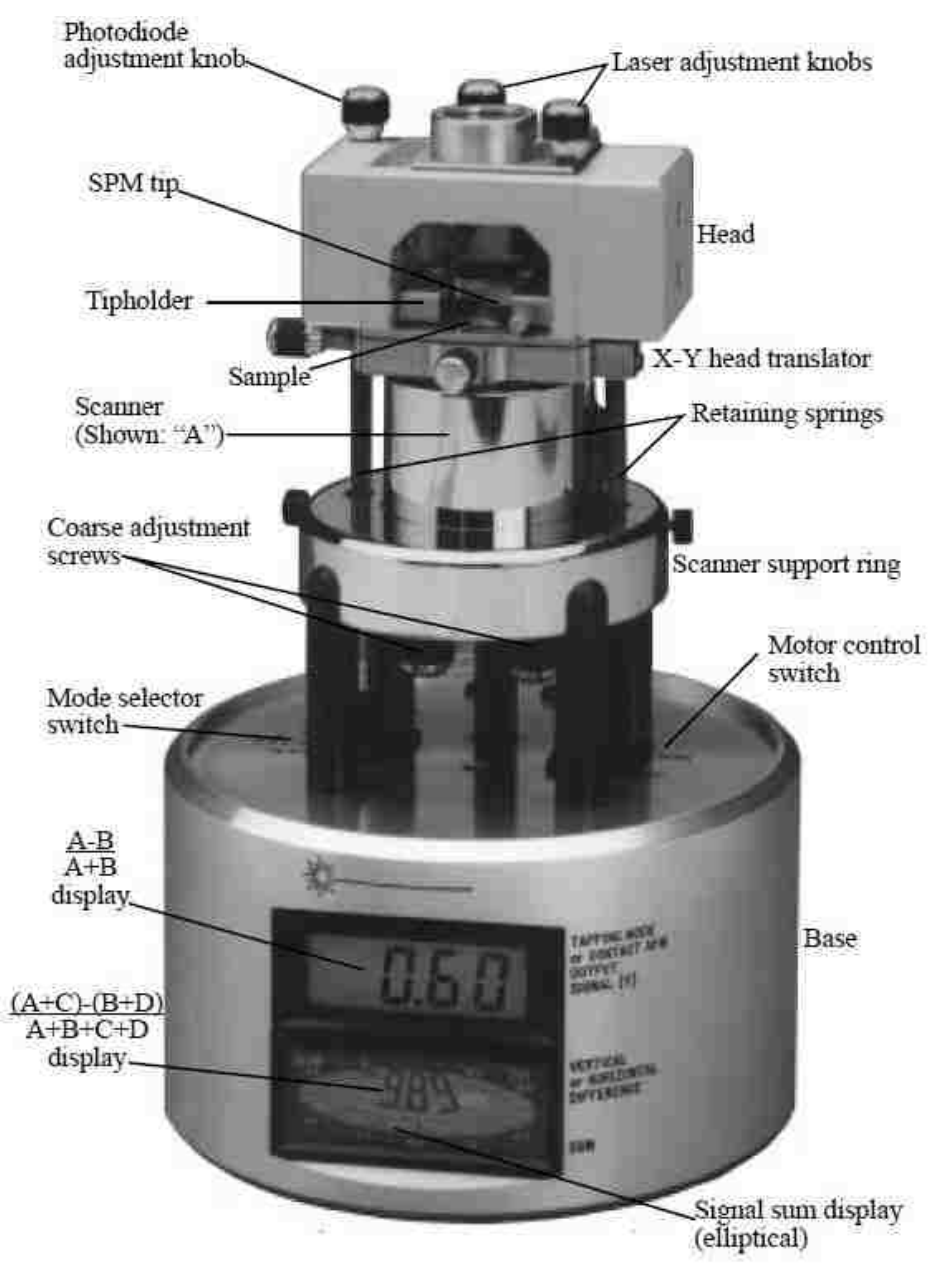
Figure A. 3. Multimode SPM [Digital Instruments Instruction Manual for SPMs, Version 4.12, Pg. 2-3]
