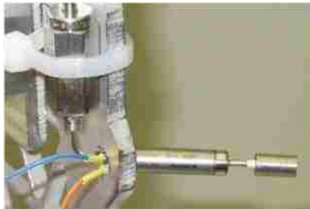
Figure B.10. Lee Company Valve with Integrated Nozzle on MR SAT Side Panel
