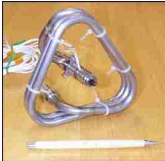
Figure 1.7. SNAP-1 Two-Phase Butane Propulsion System
