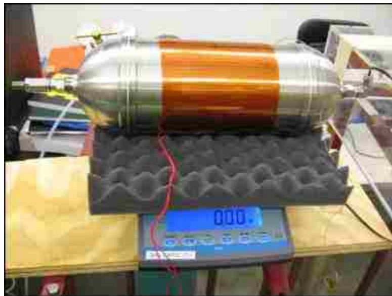
Figure 4.4. Measuring Propellant Mass in Propulsion Tank Using Scale
