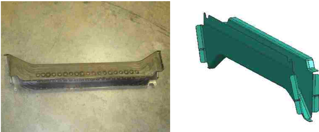
Figure 2.7. Crossing member reinforcements
