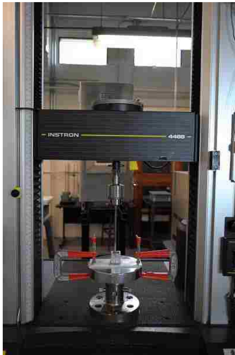
Figure 5.6. Tooth Setup for Fatigue Test in Instron 4469
