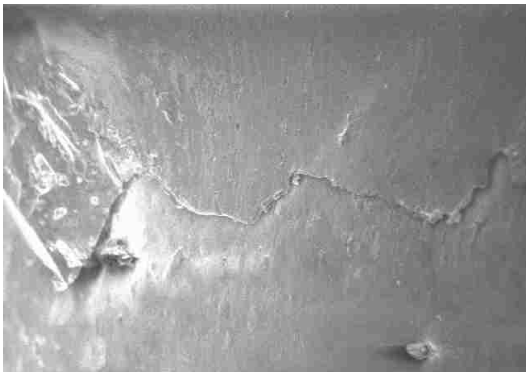
Figure 6.17. Loss of Enamel with the Formation of Cracks.
