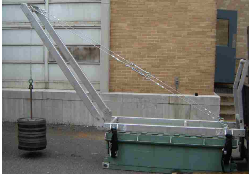
Figure 4.18: First Design of Crane System
