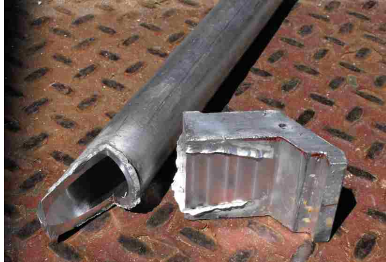
Figure 4.5: Carry Bar Prototype Failure
