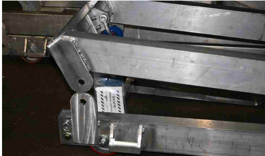
Figure 4.20: Welded Plates for Wire Rope Assembly
