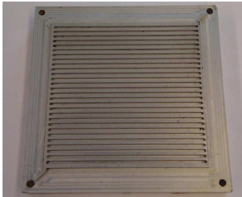
Figure 3.5. Bipolar plate compression mold with parallel flow field
