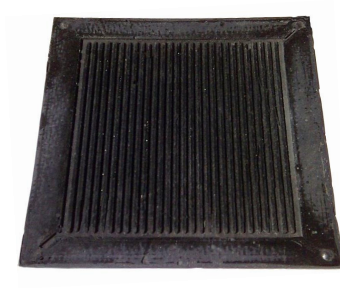
Figure 4.10. Compression molded hybrid composite bipolar plate
