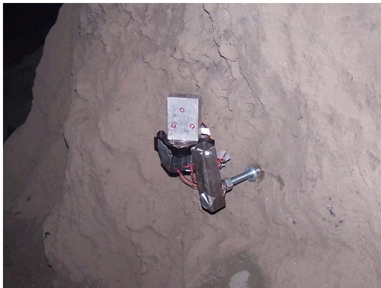
Figure 3.5: Three incidence lasers mounted directly to a rock wall.
