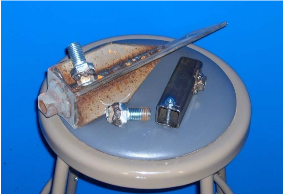
Figure 3.7: A wall mount for the target or sensor platform (left). The wall mount for the incidence laser(s) (right). Thread adapters (resting on top).
