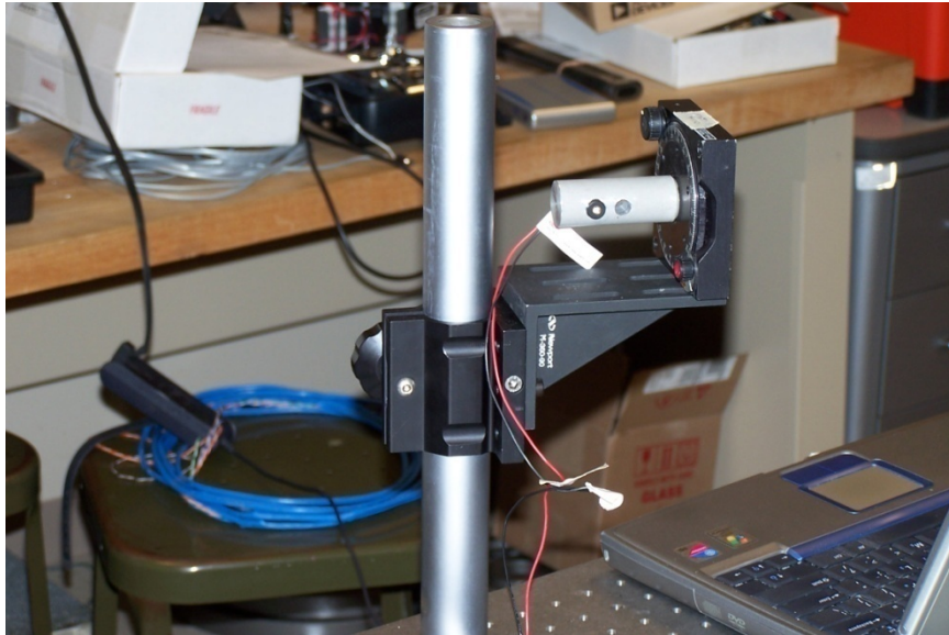
Figure 3.4: Laser diode and rotational stage mounted to an optical experimentation table in the laboratory.
