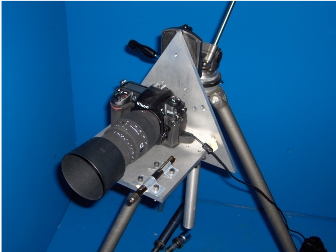
Figure 3.2: Sensor section of the HRTMM including the Nikon D200, Sigma lens, targeting laser, sensor platform, and video tripod head all mounted on a tripod.
