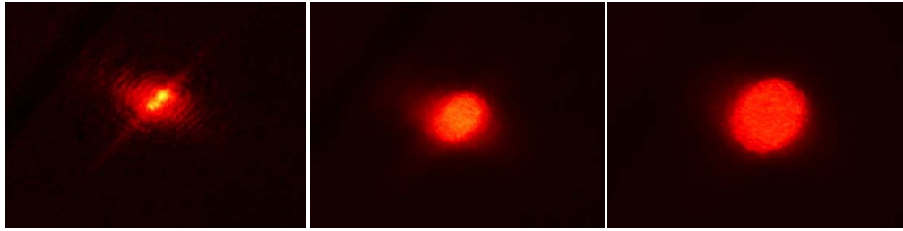
Figure 5.3: Crops of three laser spots with three different camera focus settings; in focus, approximately 30 cm out of focus, and approximately 100 cm out of focus, respectively, left to right.
