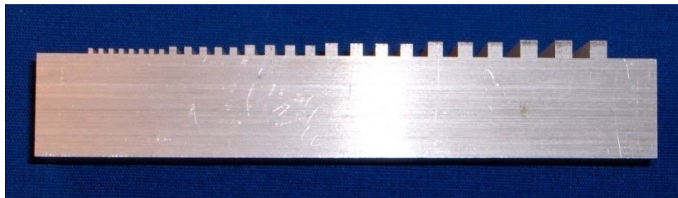
Figure 5.13: Cross-sectional view of the metal fabricated roughness target.
