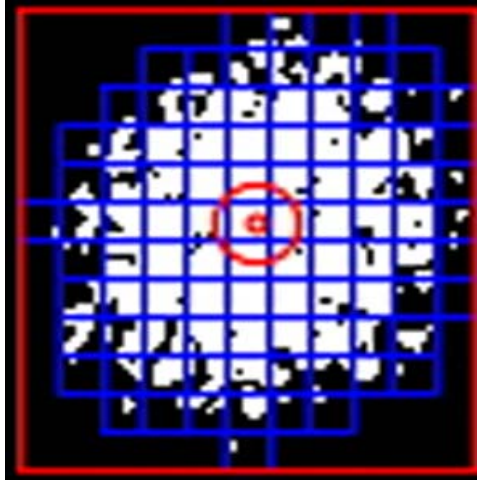
Figure 3.8: Example of a laser spot returned by the HRTMM program.
