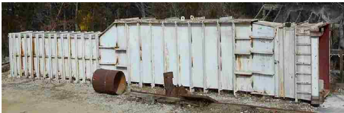
Figure 3.8: Fabricated Steel Shock Tunnel Used for Barrier Bag Testing
