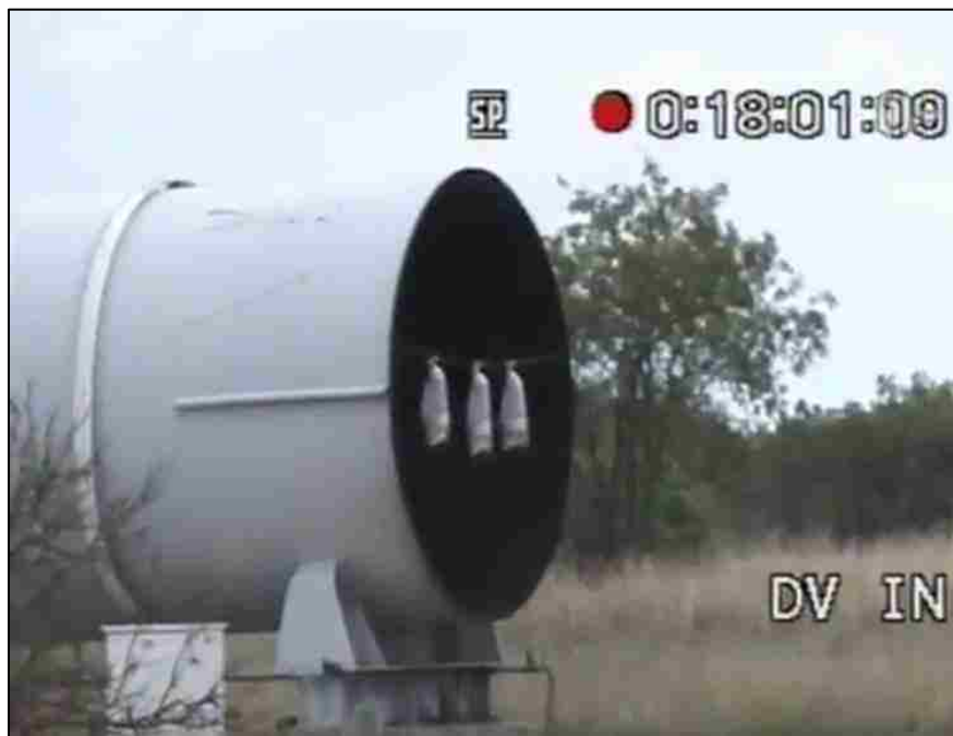
Figure 2.3: Bag Testing in Shock Tunnel at Kloppersbos Testing Facility
