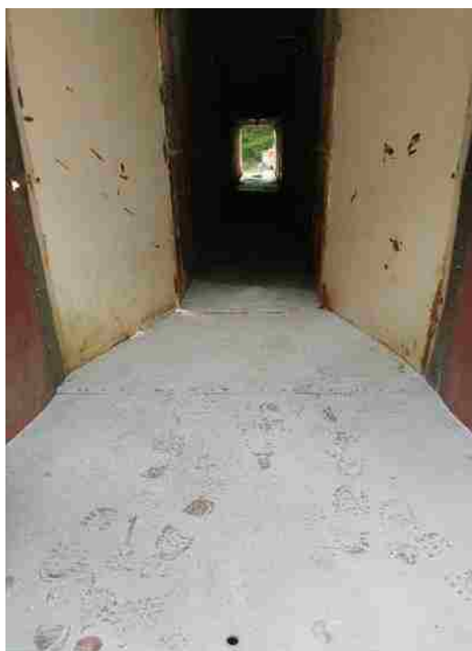
Figure C2.1: 40g C4 Test Bag Distance 35 feet
