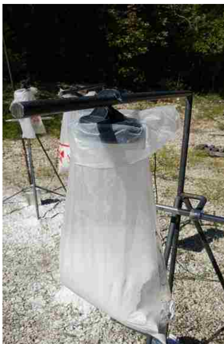
Figure C1.2: 120g C4 Test Bag Position 3 (9 ft)
