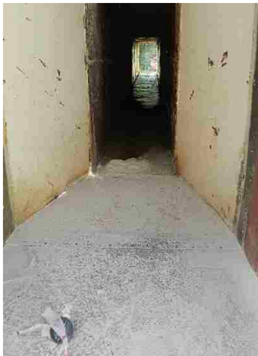
Figure C2.2: 40g C4 Test Bag Distance 39 feet
