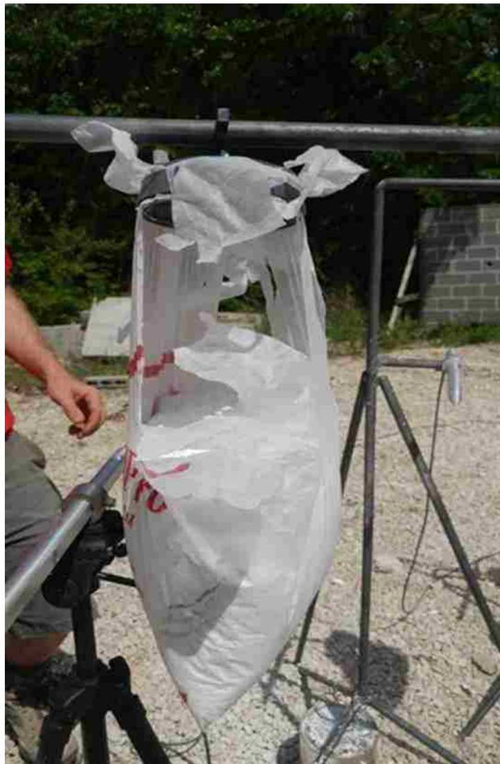
Figure C1: 60g C4 Test Bag Position 1 (5 ft)
