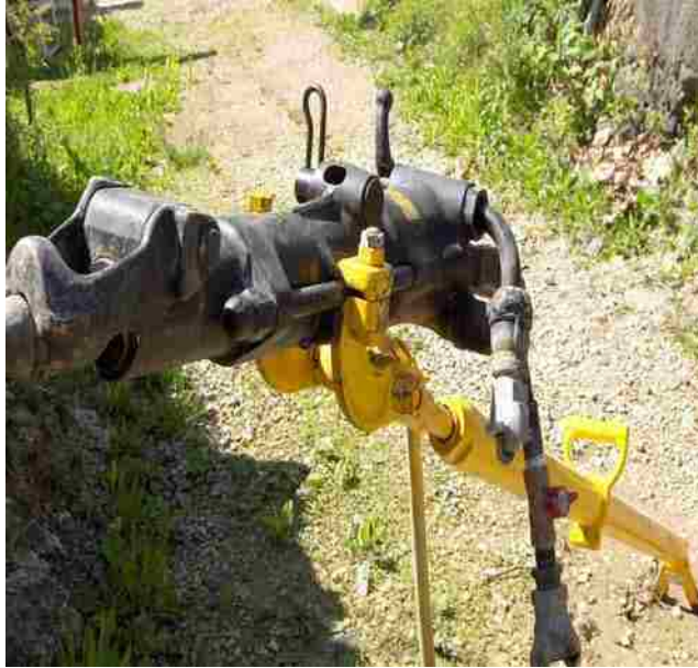
Figure 2.7. Drill Head Mounted on the Telescopic Leg.
