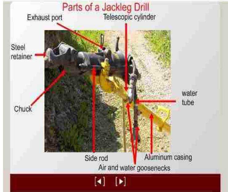
Figure 3.3. Screen View Showing Major Parts of a Jackleg Drill.
