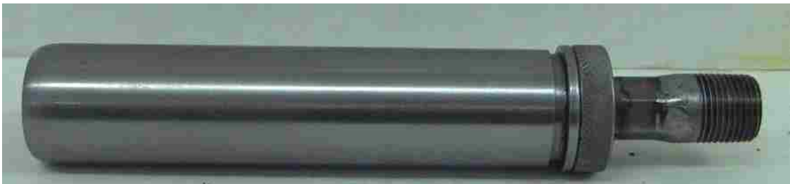
Figure 3.12. The Drill Steel Model at its Fully Collapsed State.
